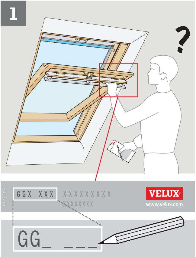
**ENGLISH:** Identify the window type and size from the window data plate. The three first letters indicate the type of the window. The next three characters refer to the size of the window.
